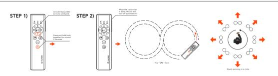
TIPS: Keep distance from magnetic interference during the calibration. We recommend calibrating Wizard outdoors. You can find the TYPHOON Wizard calibration tutorial video at www.yuneec.com/wiz-info.html
